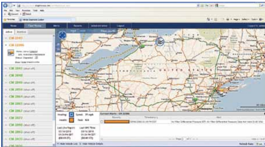
Vehicle Health Management System: In almost real-time, customers can access the Web-based interface to view the location and condition of their vehicles, as well as driver behavior. The system saves an estimated $3,000 per truck annually.
