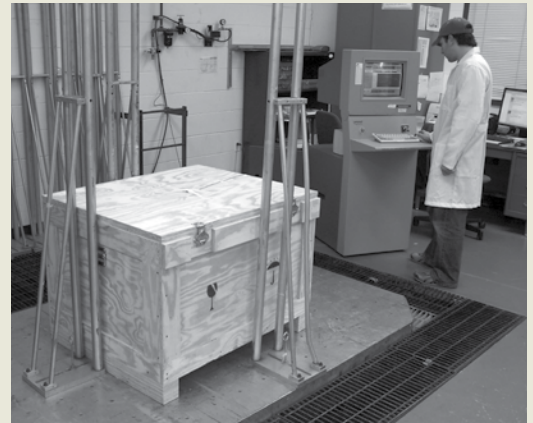
Packaging Dynamics Laboratory: Environmental testing, vibration analysis, compression, and impact assessment is conducted at the Packaging Dynamics Lab to simulate how industry partners' packaging will hold up under different conditions.
